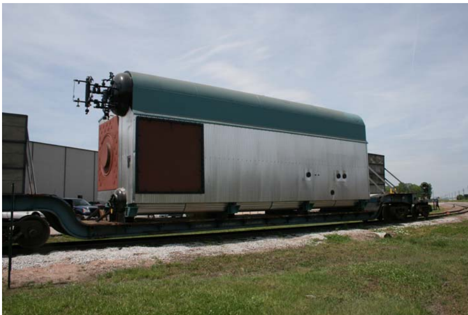
Fig 1: (Addendum) Custom designed 150,000 lb/hr Nebraska D Type superheated steam boiler engineered for future low emissions with finned tube convection bank (shown ready to ship via railcar).
