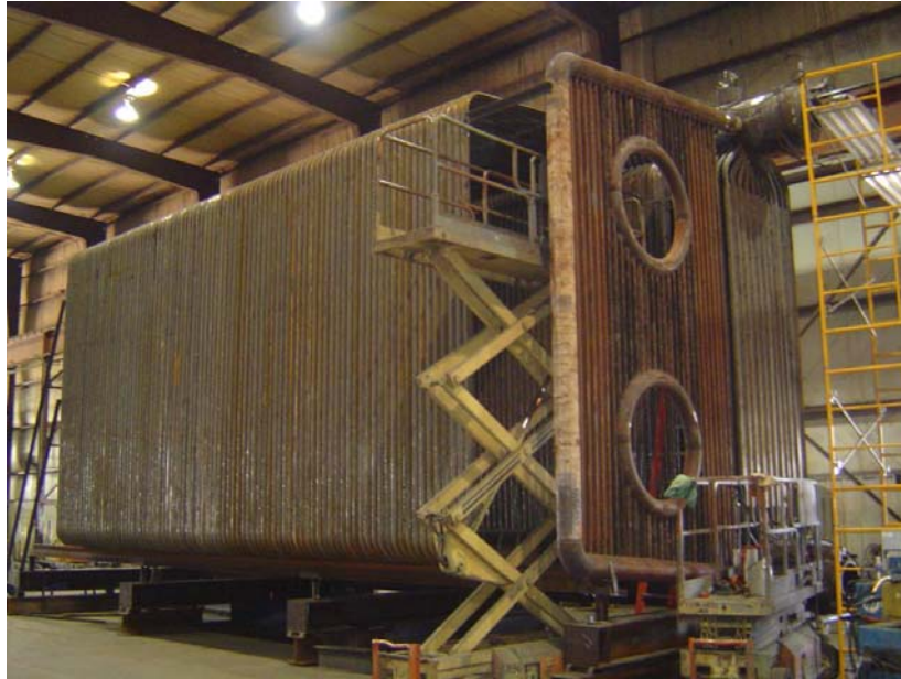
FIG: 6: (Addendum) 100% water-cooled membrane furnace design avoids costly refractory maintenance. Unit shown is a 426,000 lb/hr design during manufacture.
